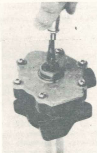
Filling the oil channels by turning the pump shaft.
