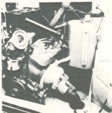
Oil tank and oil pump
