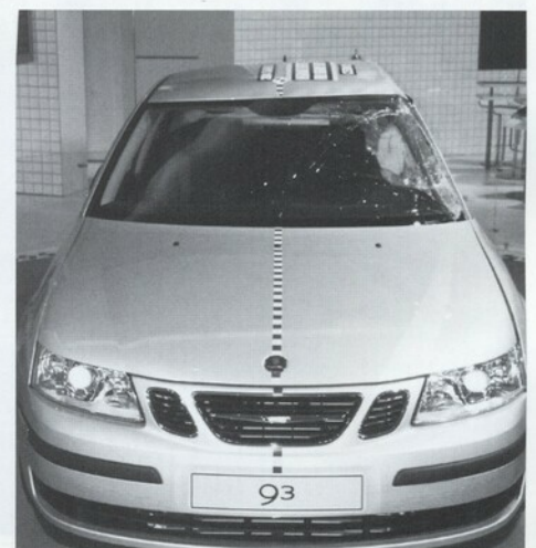
Thoroughly crunched 9-3. Note the lack of deformation on the passenger side of the vehicle in the front view photo.
