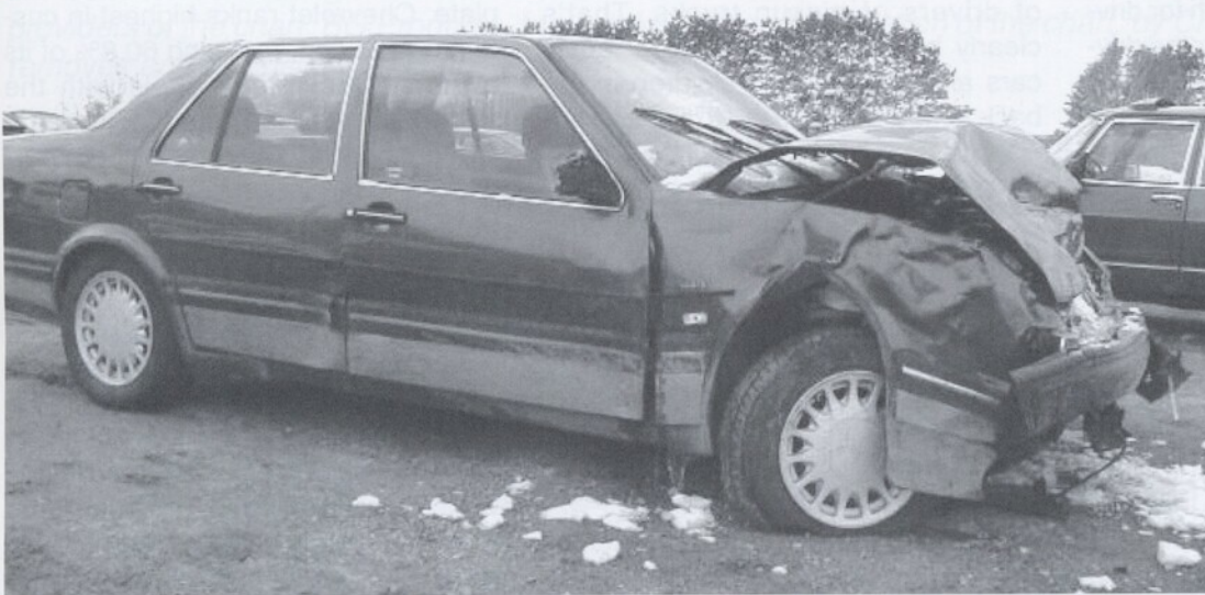
Daughter-in-law hit head-on on a two lane road. The roof is buckled, even the rear door has buckled near the bottom. The air bag deployed and she had the safety belt on. Total injuries were a bruised knee and bruised shoulder from the seat belt. Proof positive that active safety in practice saves lives and injuries. Even when you can't avoid the crash, you don't have to be crunched. Photos by the author.
