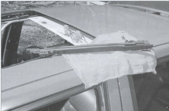
Support arm out of the track
