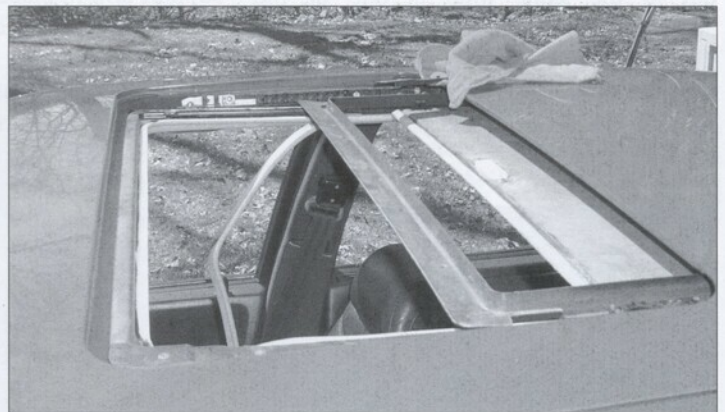
Sunshade and frame in position.
