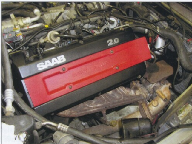
Saab DI Cassette installed on a Classic 900.
