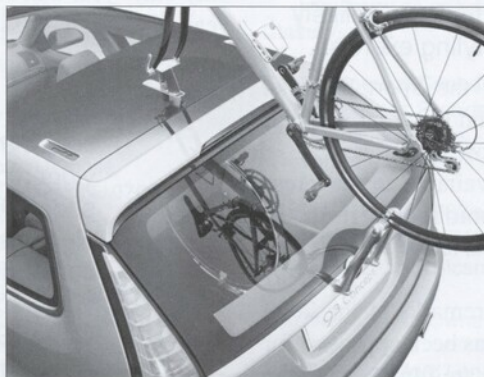
Recessed load points take the place of roof racks.
