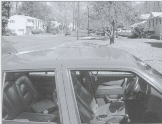
A steel sunroof was standard equipment on 1991 9000S and Turbo models in the USA.
