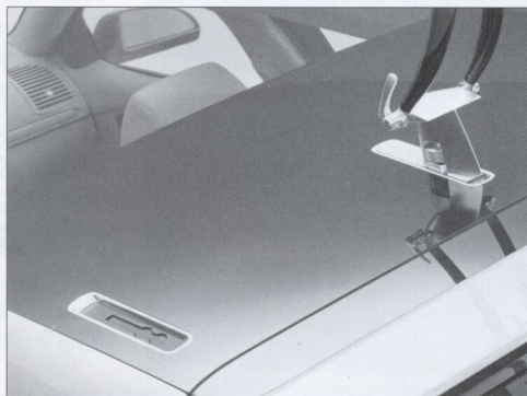
Close up view shows a bicycle mounting "foot" installed in one of the load points.
