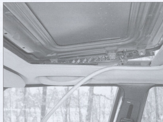
Remove trim from around sunroof opening.
