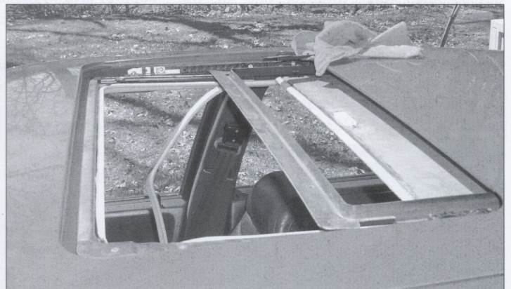
Sunshade and frame in position.
