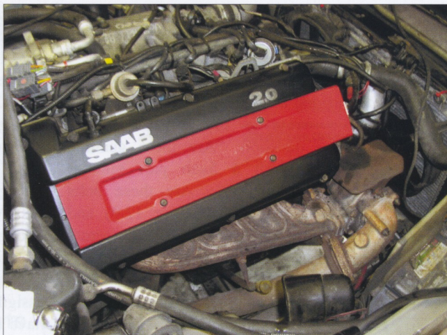
Saab DI Cassette installed on a Classic 900.
