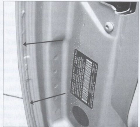
Vinyl seam sealer on the lap seam of the driver's door. Photo by author
