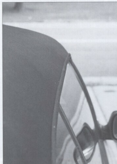
The convertible top “rain gutter” is essentially a rolled seam.
