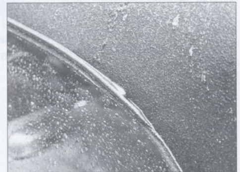
The “rolled seam” rain gutter is extremely effective in channelling water.
