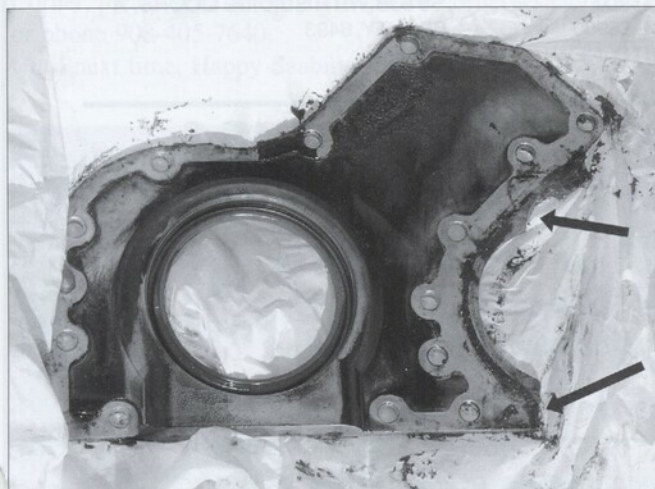
Broken gable plate. Arrows point to fracture surfaces.
