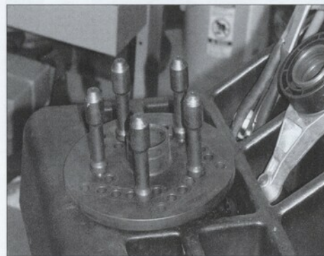
Conical pins clamp the wheel using the lug bolt holes.
