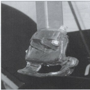
"Bead stretcher" arm is tipped with a no-scratch plastic foot.
