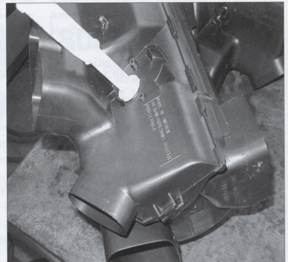
9 3 S Heater box with rod in place. Notice: For you Saab fans, this isn't a GM part! It says "Made in Sweden" in English so even I can read it.
