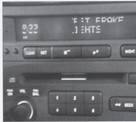
9 5 SID panel shows the segments failing. The display should say, "Test Brake Lights" plainly and the time at 9:22
