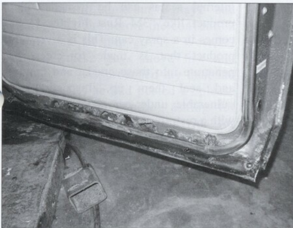
Door bottoms are especially susceptible if drains are not clear.
