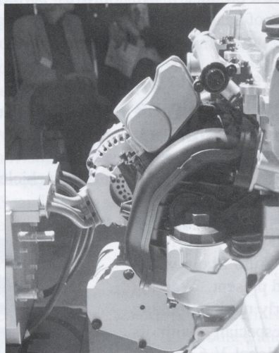
A rear view shows the massive electrical wiring between the controller module and the combination starter/alternator.
