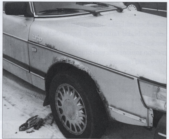
When surface rust is this bad, there is often structural damage as well.
