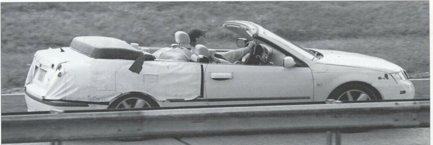
Captured! 2004 Saab 9 3 prototype undergoing testing. The top cover is obviously not "production". The most striking feature to be seen from this disguised prototype is the straight line rising wedge shape of the "greenhouse". Prototype is sufficiently developed that the "Onstar shark fin antenna" is mounted to the trunk lid. Photograph by Hans Lehman/Hidden Image.
