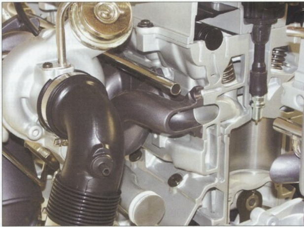
Cut away showing the Saab head, pistons, turbo.
