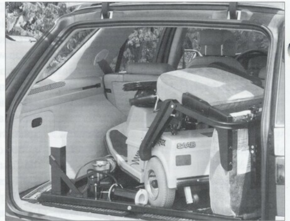
Electric scooter and lifting winch secured in the back of Carrellas' 9 5 SportWagon
