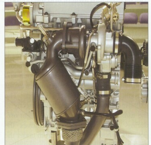
Rear view showing the turbocharger and the close coupled catalyst.
