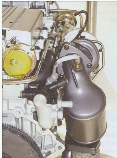
Close coupled exhaust catalyst, cam driven vacuum pump, thermostat housing.
