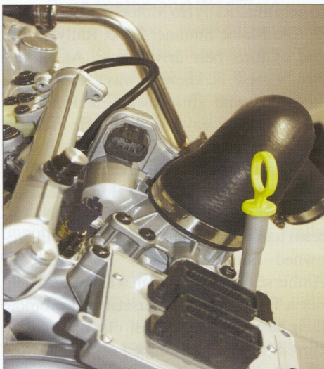
Drive by wire throttle body, engine management computer.
