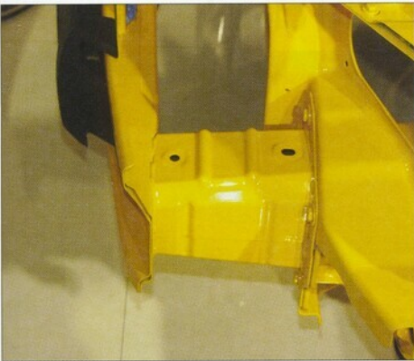
“Crash box” protects the unibody from damage in moderate level impacts.
