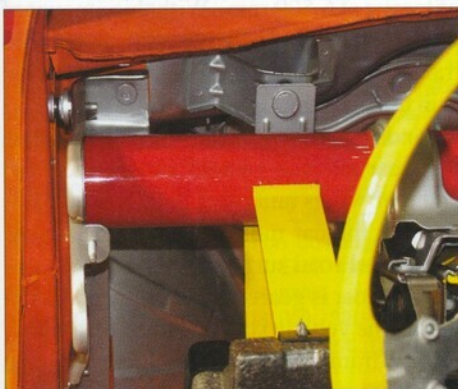
A sturdy steel tube supports the dashboard
