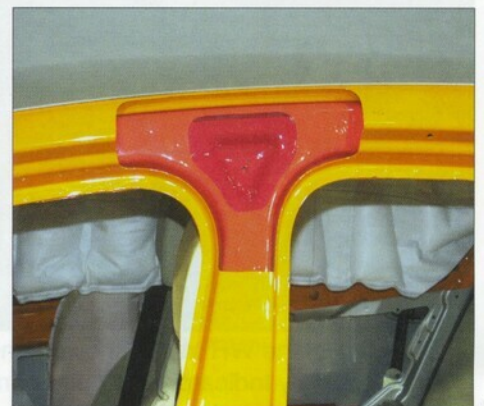
Triple steel structure of the "B" pillar.
