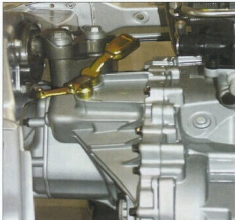
Cable shift levers and "pendulum" mount. Note weighted lever for proper "fore-aft" shift lever feel. design. The gears, bearings, shafts, and case are identical to the older gearbox. The synchronizers in the 5-speed box are now made from carbon fiber, and are similar to the friction material used in Formula 1 race car brakes. Widmark told us that when these cars are scrapped at the end of their lives, the
