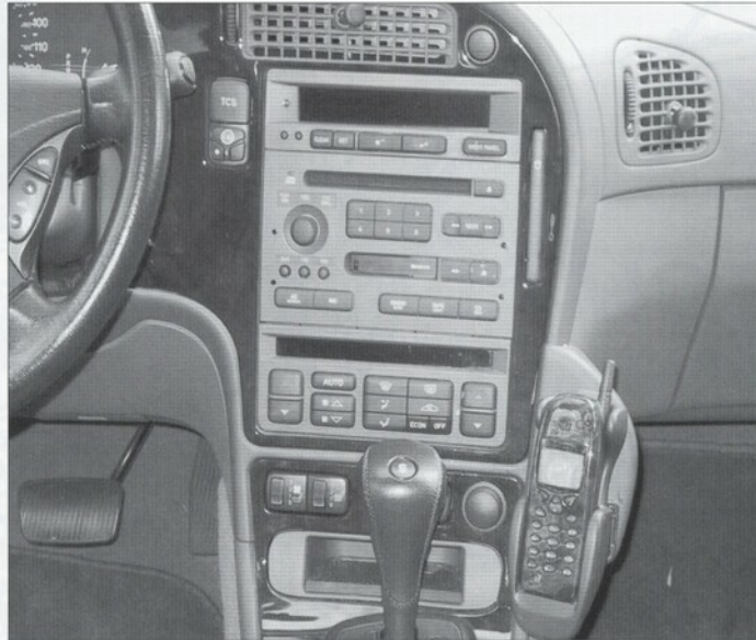
UHLtronics Triad allows a Nokian cell phone to be operated hands free using the OnStar microphone and Saab audio.
