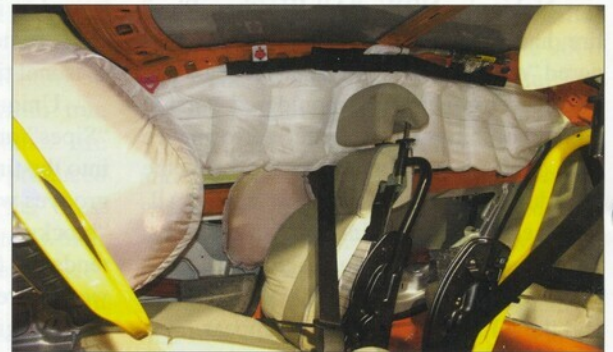
Dashboard and steering wheel, side curtain, and seat mounted torso "air bag" restraints.
