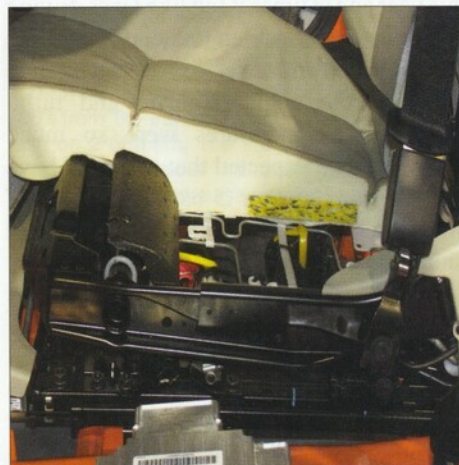
Resilient foam prevents “submarining” and prevents injury from seat structure.
