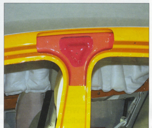
Triple steel structure of the "B" pillar.
