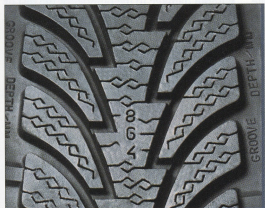
Close up of the WR tread, showing the Driving Safety Indicator (DSI) numbers molded into the tread and the geometry of the "Haka Siping".
