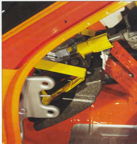
Resilient foam knee pad is supported by collapsible steel support.
