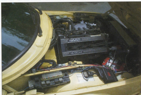
16 valve Twin Cam "S" engine mounted in Tom Letourneau's 1979 99.
