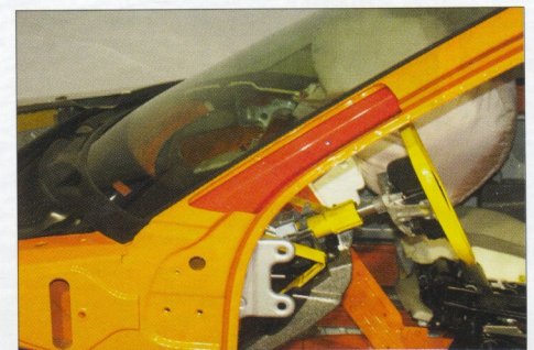
Twin tubular A-pillar structure is much stronger than a single tube structure.
