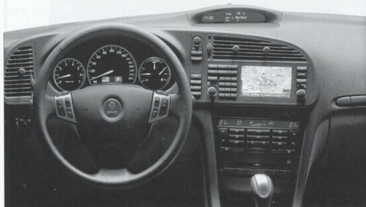
The cockpit layout and design clearly descend from the Classic 900. The block of buttons to the left of the navigation screen operates the integrated phone.
