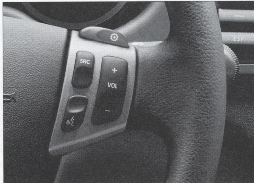
Steering wheel mounted shift paddle, along with (on the right) audio volume and source, and cell phone microphone controls.
