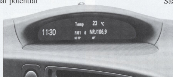
Saab Information Display (SID) is relocated to the top center of the dash top for easier viewing while driving.
