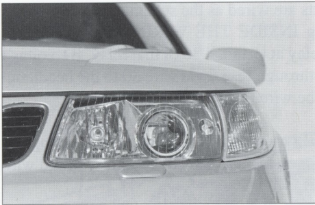
2002 Saab 9 5 with optional Xenon electric arc discharge headlights Photo courtesy of Saab Automobile AB
