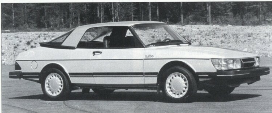
Prototype of a removeable hard top. This top was not put into production because the projected total sales of Saab convertibles was just 3000!
