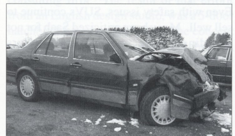
A totally collapsed engine compartment, a totally intact passenger compartment.
