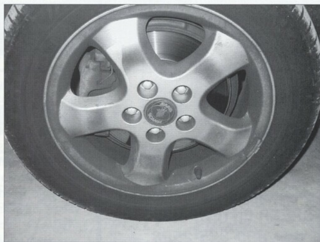
The dusting shown on this 9 5 front wheel is typical of the OEM semi-metallic pads used on European cars.
