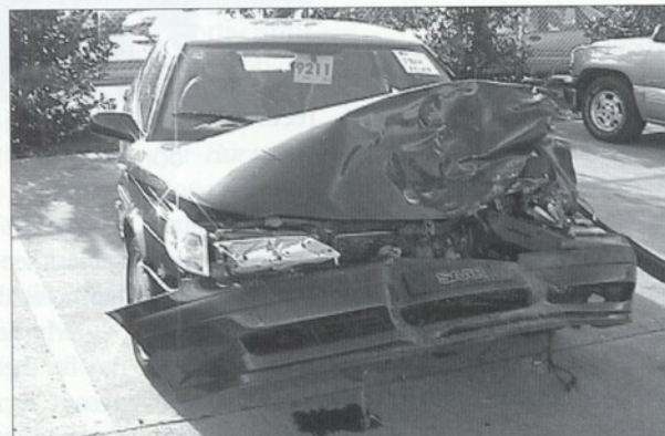
The upper front structure absorbed the impact forces.
