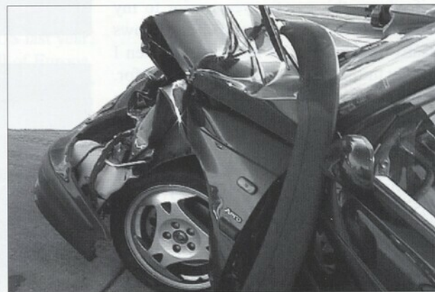
Crumpled and mangled from a classical offset frontal collision.
