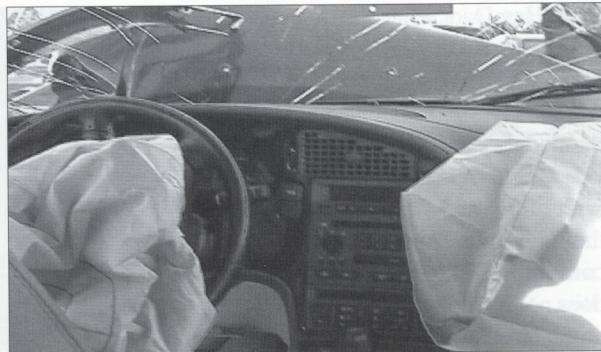
Stress cracks in the glass result from the body distributing the impact forces.
