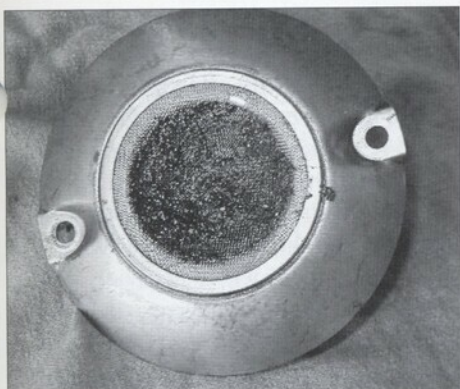
A clogged oil pick up screen from a 2.3 liter "900S". Photos courtesy of Chuck Andrews
