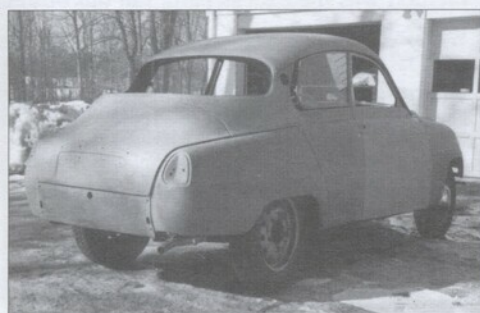
Body work complete and sprayed with primer, ready for the finish coat.
