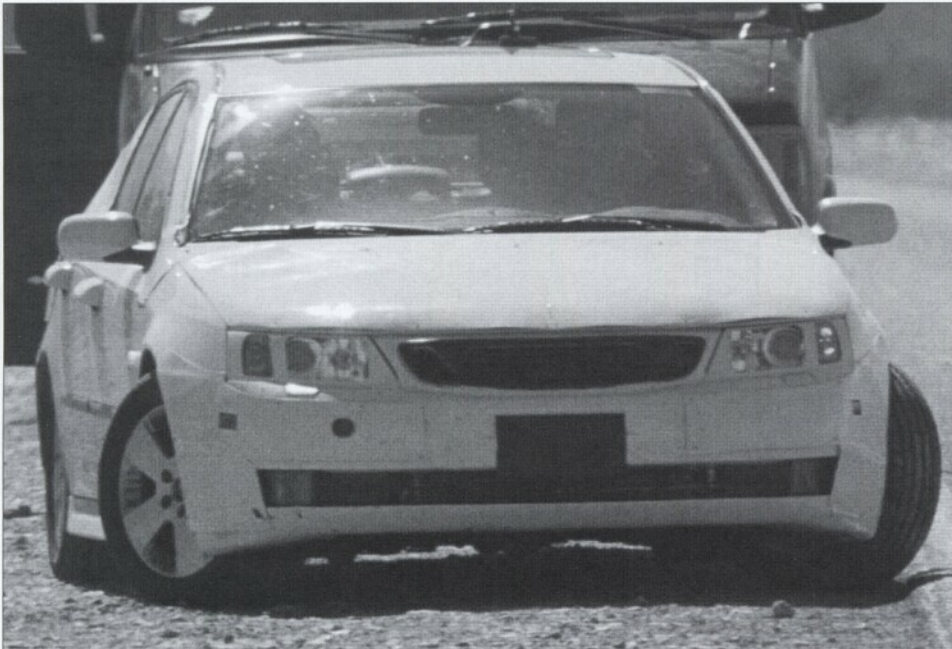
Front view of the new 9 3 undergoing testing in the Southwestern US. The hood and front bumper are masked, along with the area in front of the side view mirror. Note the rising wedge side character line and flat sides.
