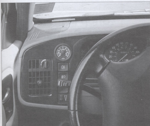
A calibrated pressure gauge is a perfect fit in the opening for the headlight switch.
