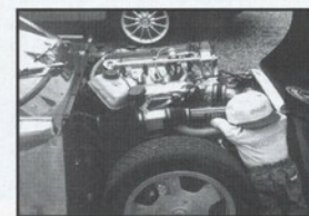
2nd Modified: 1968 Sonett III 16 valve Turbo conversion. John Plakey
