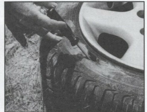
This won't be fixed. Note the absence of "shredding", despite "running on the rim" at high speed.
