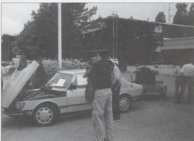
Leave it to those wacky Finns - a wood-burning stove follows this 99 around at all times, creating a swamp gas-like mixture that powers the standard B-motor.
