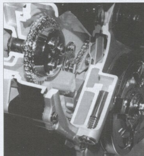
The water pump drive and oil pressure relief valve are seen in this view.
