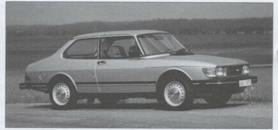
The Saab 90 combined the front section from the 99 with the 900 sedan rear section.
