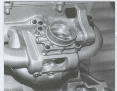
The drive-by-wire throttle assembly shows no trace of a mechanical linkage.
