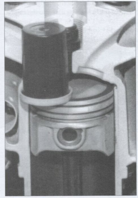
The piston in the SVC engine is barely half the diameter of the Global 4
