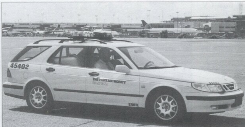
Saab 95 Runway Friction Tester
