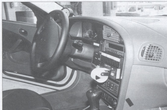
Driver's Cockpit showing the computer and data printer in place of the Saab radio.
