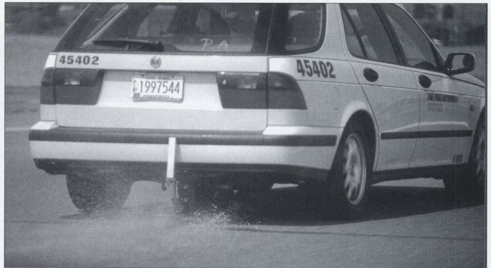
Water sprays as the Runway Friction Tester goes through a runway calibration test.
