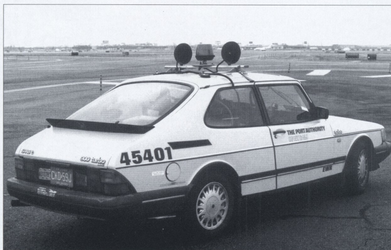
Previous generation Runway Friction Tester built into a 1987 Saab Turbo.
