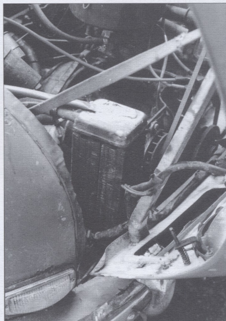
Heater core added to a Saab 96's cooling system, mounted to the right of the water pump/generator.
