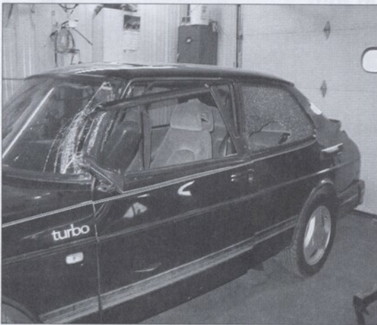
87 900T showing damage caused by semi trailer at shoulder level.
