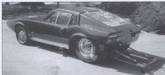
Wheelie bars and massive rear slicks show that this is no ordinary Sonett.
