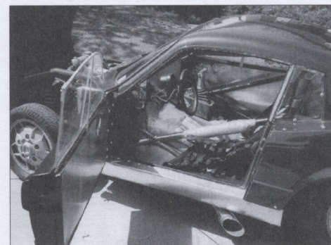
The minimalist interior shares space with the tube frame.
