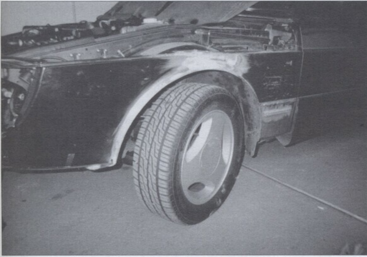
Figure 3: Front fender being cut in at All Car Auto Body, San Mateo CA.
