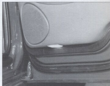
Figure 12. Door mounted courtesy light and weatherstrip.
