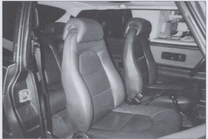
Figure 5: Interior. Front and rear seats replaced with a set from a 1988 SPG.
