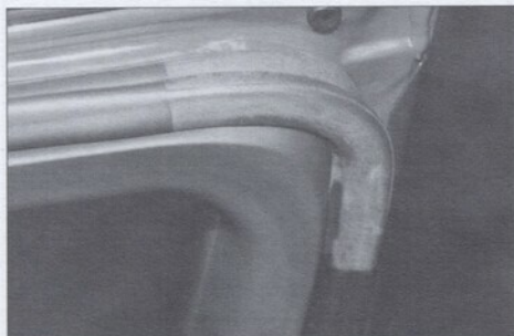
Figure 13. Teflon wrapped weather strip corner detail.
