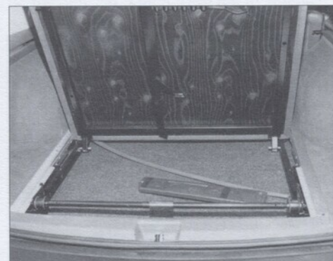
Figure 16. Roll out load floor raised to show under-floor storage.
