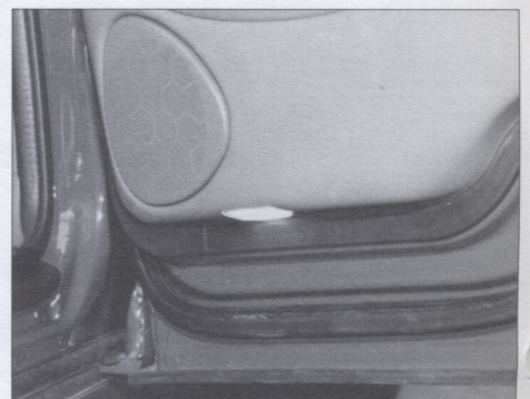
Figure 12. Door mounted courtesy light and weatherstrip.
