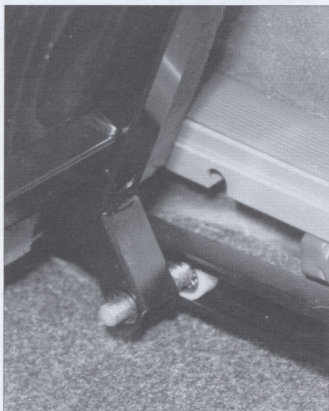
Figure 17. Detail of load floor roller.
