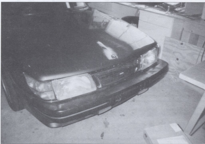
Figure 1: Poorly fitted hood, headlights, grill and side directional markers. The '86 SPG should have the headlight/light in bezel but someone tried to install '87> headlights and grill.
