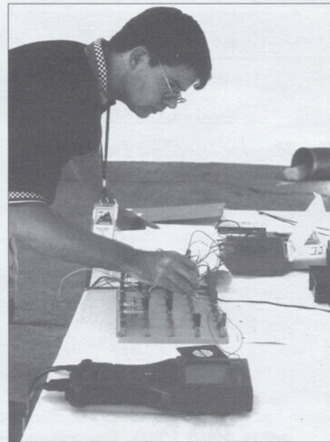
Building up part of the dashboard wiring circuit using a "breadboard" and a "DICE" dash computer.
