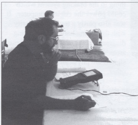
Using the Tech 2000, a technician can diagnose the car using stored data. The car need not be present.
