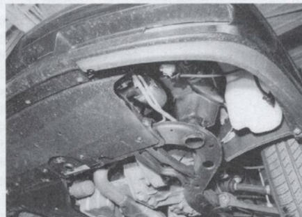
Figure 3: Front Subframe. Note frame to body mount, suspension pivot mounted to frame side, and fog lamp connector.
