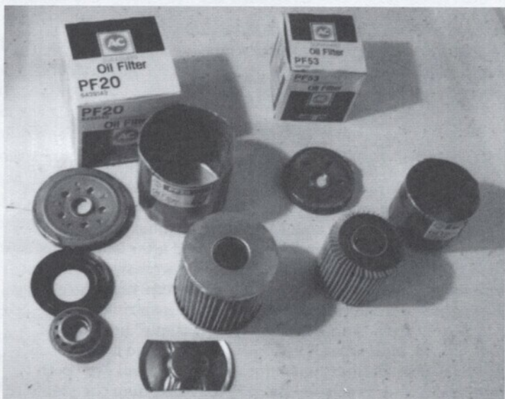
Figure 4: AC filters. In small filter, element fits against filter case. Black rubber lower end plate serves as anti-drain valve, pressed against baseplate by internal components. In large filter, "flying saucer" houses bypass valve mechanism - a spring loaded rubber diaphragm. Anti-drain valve is similar to small filter.
