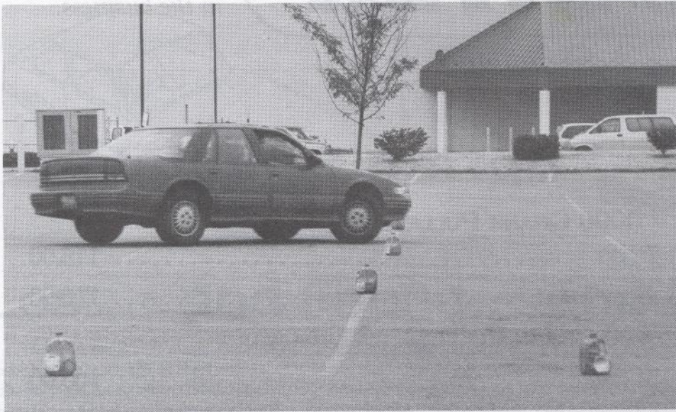
"Modified Slalom" view from the "starting gate." Driver must negotiate the course repeatedly, which requires crossing the center line at close to right angles. This is not his Father's Oldsmobile.
