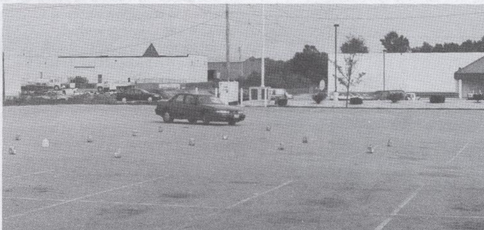
Bottom: Maximum braking exercise is best performed on wet, "sealed" asphalt using a non-ABS equipped test vehicle.
