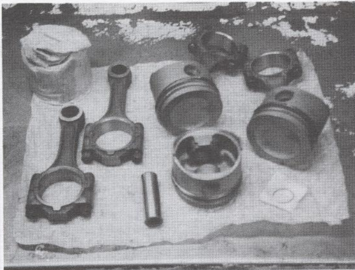
New standard size pistons were installed on the old connecting rods.
