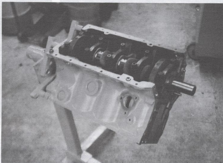
Step one of reassembly, the cleaned up crankshaft is installed into the cleaned up and freshly painted engine block.
