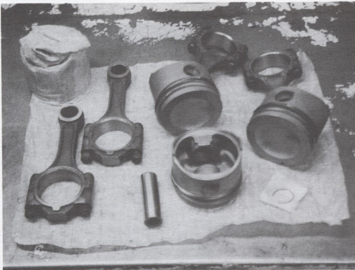
New standard size pistons were installed on the old connecting rods.
