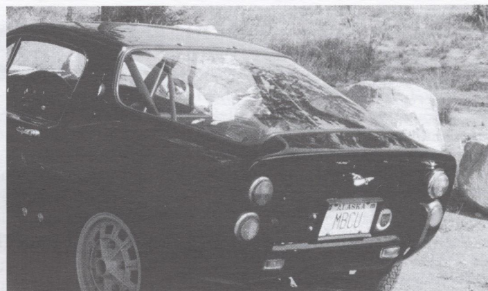
The compound curve rear windows for the Sonett II/V4 are no longer available, so be very careful when removing.
