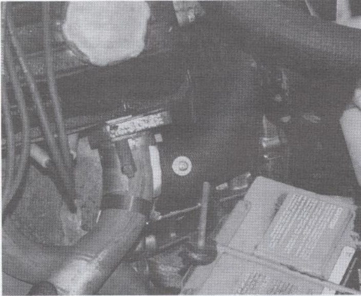
A simple duct was set up to direct warm air from the headers into the air cleaner.
