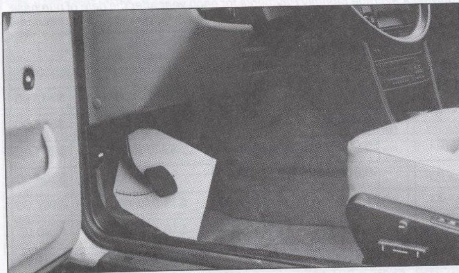
Template made of foamcore fits tight against the clutch pedal.
