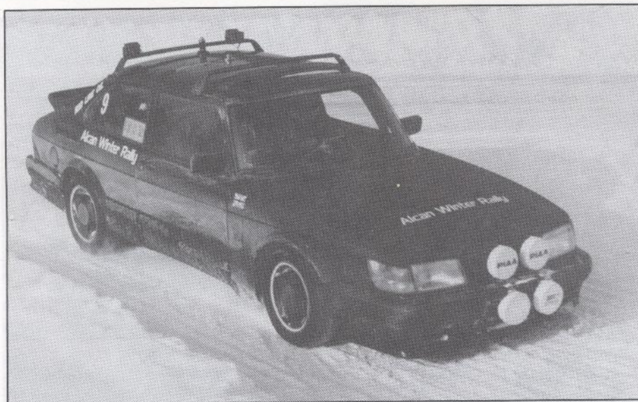
Blackbird at the Quesnel Solo. The roof rack carries extra tail and brake lights.
