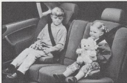
Integrated child booster seats are an option on the rear "Saab Safeseat" system. The 40/60 split seat features three-point harnesses for three seating positions.
