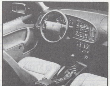
Cockpit styling of the instrument panel has been refined. All controls are within easy reach. The Black Panel illuminates only the speedometer unless another system needs to inform the driver.
