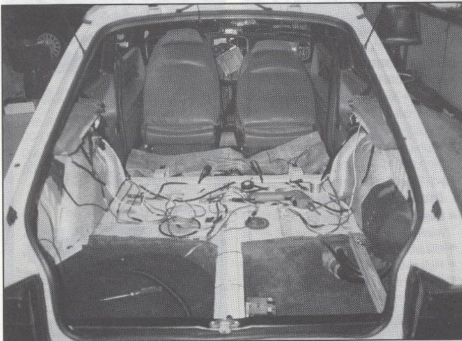
All of the interior had to be removed for installation of wiring and components.
