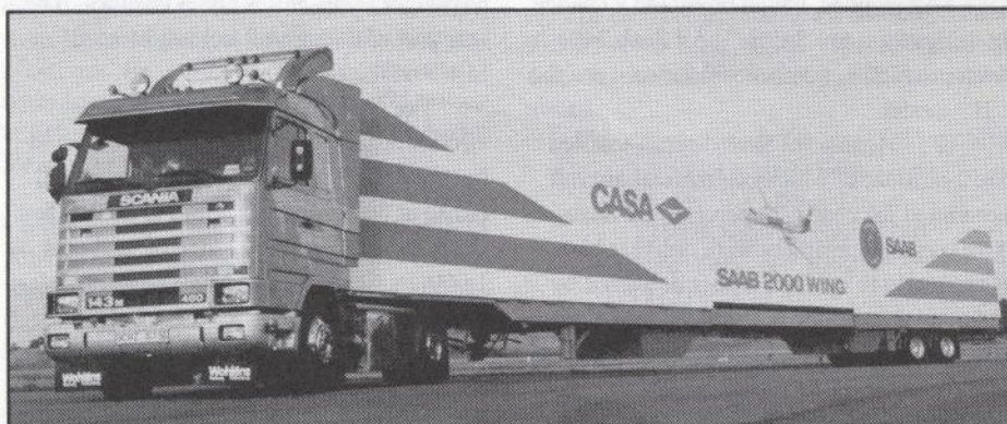
The wing for the Saab 2000 is transported from Spain in this special trailer.
