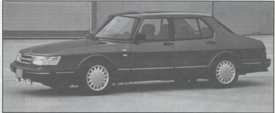
New 15-spoke alloy wheels are the most visible difference on the 1992 900S
